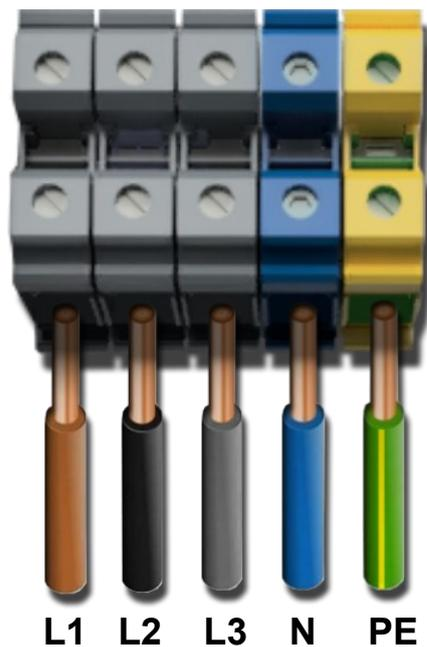
Connect Power Supply Cable three phases L1; L2; L3 to three separate wire terminals. (Grey color wire terminal)
