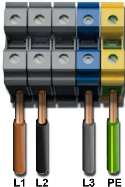
For TN 3-Phase: connect L1 to charger's Phase 1. Connect L2 to charger's Phase 2. Connect L3 to charger's Neutral.
